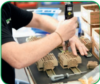
Terminal rail mounting / assembling
